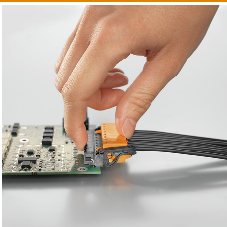
Self-locking Immediately on plugging in
