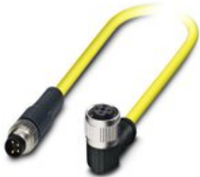
Sensor/actuator cable, 4-position, PVC, yellow, Plug straight M8, on Socket angled M12 SPEEDCON, coding: A, cable length: 0.5 m
