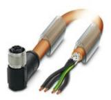
Power cable, 4-position, PUR halogen-free, orange RAL 2003, shielded (Advanced Shielding Technology), free cable end, on Socket angled M12, coding: S, cable length: 1.5 m, for AC current up to 12 A/690 V
