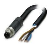
Power cable, 4-position, PUR halogen-free, black-gray RAL 7021, Plug straight M12, coding: L, on free cable end, cable length: 5 m, For direct current up to 12 A/63 V
