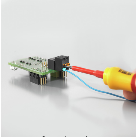
Operating safety Through PUSH IN connection system
