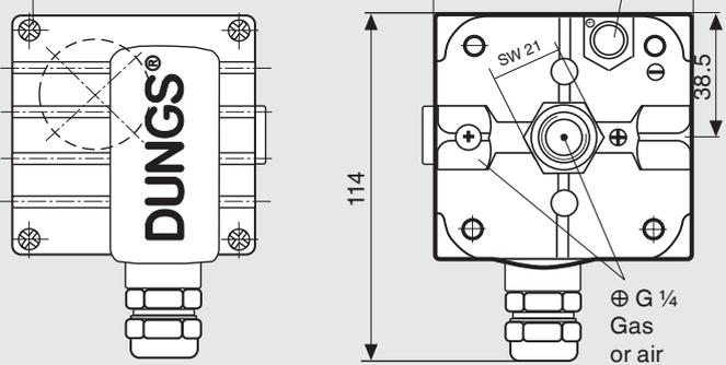
**Mounting positions** (observe the change of the switching point if mounting position differs from standard)
