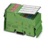
Inline, Digital output terminal, Digital outputs: 8, 24 V DC, 500 mA, connection technology: 4-conductor, transmission speed in the local bus: 500 kbps, degree of protection: IP20, including Inline connectors and marking fields, connectors numbered individually
