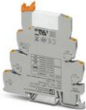
PLC-INTERFACE, consisting of PLC-BPT.../21 basic terminal block with Push-in connection and plug-in miniature relay with power contact, for mounting on NS 35/7,5 DIN rail, 1 changeover contact, input voltage 24 V DC
