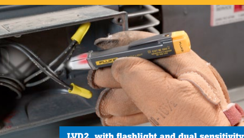
LVD2, with flashlight and dual sensitivity
