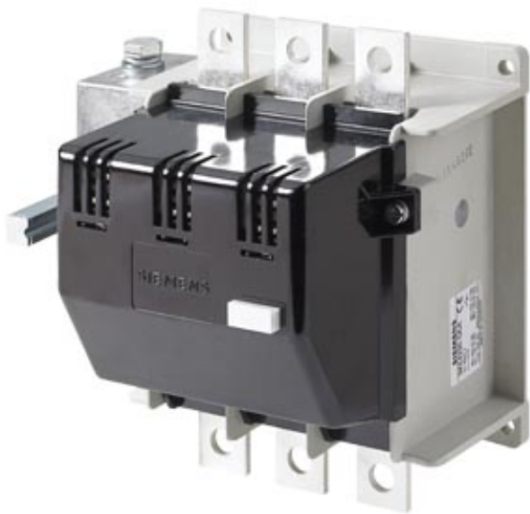
SWITCH DISCONNECTOR 3-POLE I=1000A, U=690V, FRONT ROTARY OPERATING MECHANISM WITHOUT HANDLE WITH TIN-COATED CONTACTS
