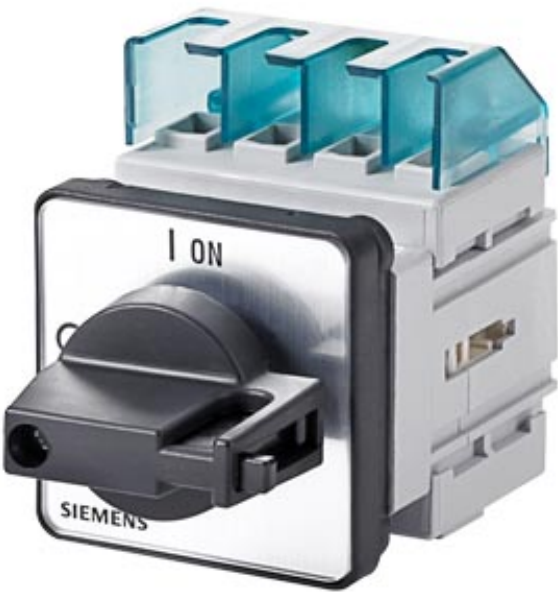
4-P. MAIN CTR./EM.-STOP SWITCH IU=16, P/AC-23A AT 400V=7.5KW FRONT MOUNTING 4-HOLE MOUNTING KNOB-OP. MECH. BLACK
