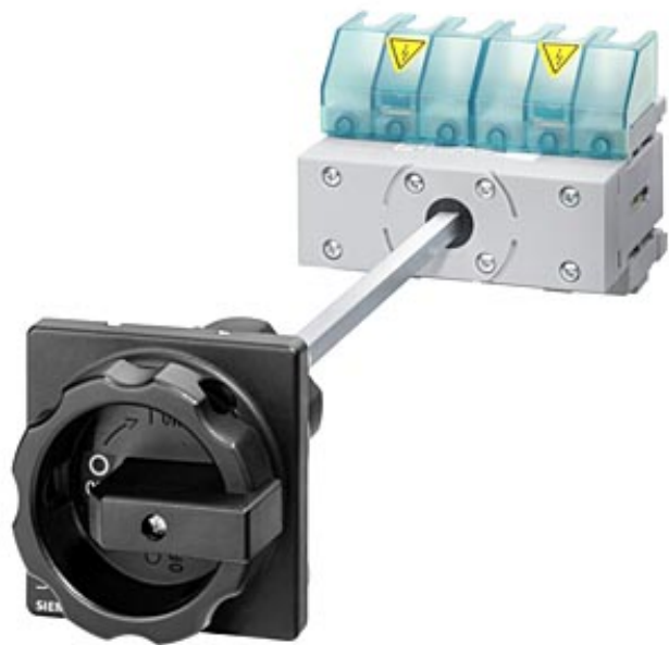
MAIN SWITCH 6-POLE IU=25, P/AC-23A AT 400V=9,5KW BASE MOUNTING DIN-RAIL- MOUNTING/ TWO-HOLE MOUNTING
