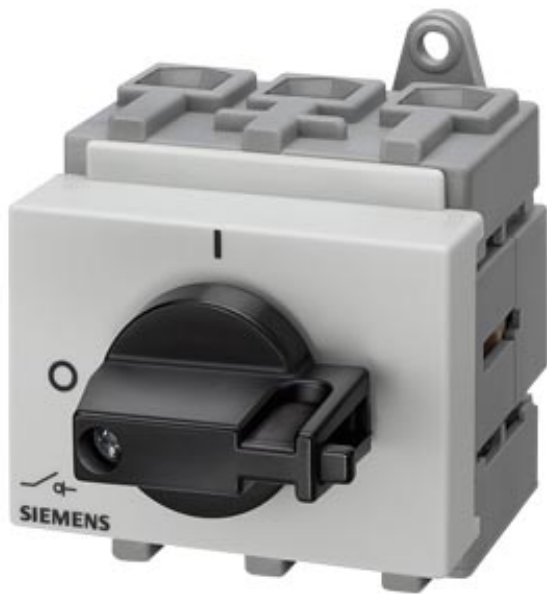
MAIN CONTROL SWITCH 3-POLE IU=25, P/AC-23A AT 400V=9,5KW BASE MOUNTING MOUNTING RAIL/TWO-HOLE MOUNTING KNOB BLACK
