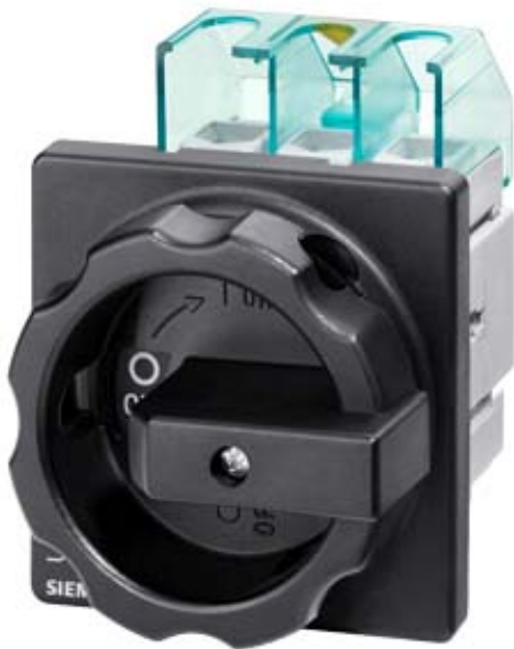
MAIN CONTROL SWITCH 3-POLE IU=25, P/AC-23A AT 400V=9,5KW FRONT MOUNTING CENTRAL-HOLE MOUNTING ROTARY ACTUATOR BLACK
