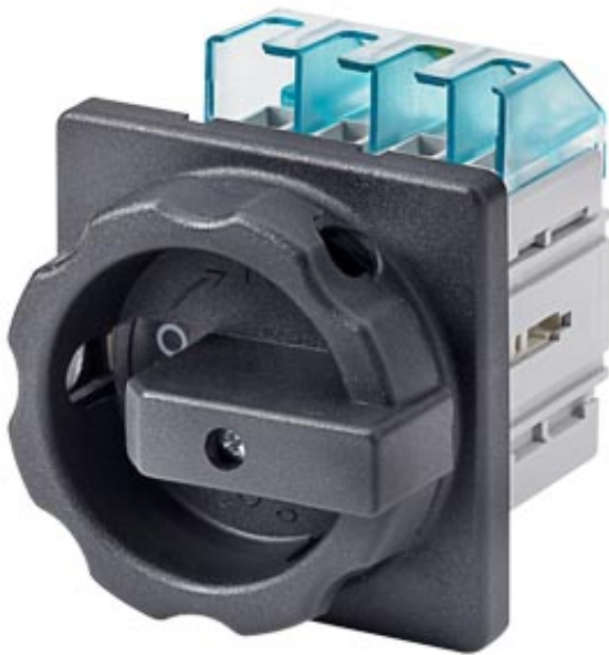
MAIN CONTROL SWITCH 4-POLE IU=25, P/AC-23A AT 400V=9,5KW FRONT MOUNTING CENTRAL- HOLE MOUNTING ROTARY ACTUATOR BLACK
