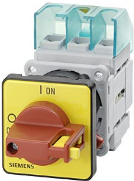
MAIN/EMERG. STOP SWITCH 3-POLE IU=32, P/AC-23A AT 400V=11.5KW FRONT MOUNTING FOUR-HOLE MOUNTING KNOB RED/YELLOW (EMERG. STOP)
