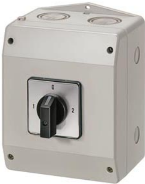
CHANGEOVER SWITCH 3-POLE IU=32, P/AC-23A AT 400V=11,5KW 2 N-TERMINAL MOULDED- PLASTIC ENCLOSED, IP65
