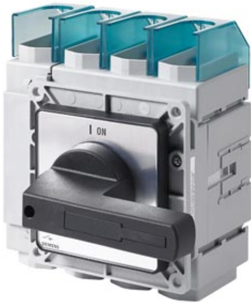
MAIN SWITCHES 4-POLE ROT. OPERAT. MECH. BLACK IU=160A P/AC-23A BEI 400V=75KW FRONT MOUNTING 4- HOLE MOUNTING
