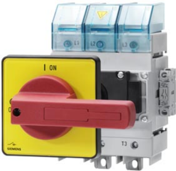
MAIN SWITCH 3-POLE FLOOR MOUNTING KNOB- OPERATED MECHANISM RED/ YELLOW (EMERG. STOP) IU=160A P/AC-23A AT 400V=75KW
