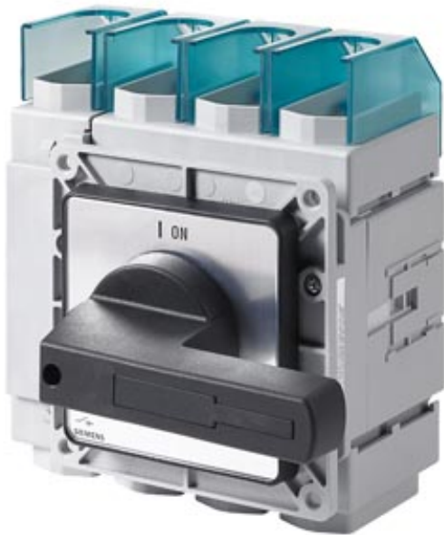
MAIN SWITCHES 4-POLE ROT. OP. MECH. BLACK FLOOR MOUNTING IU=250A P/AC-23A AT 400V=132KW 4 -HOLE MOUNTING
