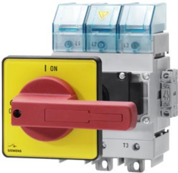
MAIN SWITCH 3-POLE FLOOR MOUNTING KNOB-OPERATED MECHANISM RED/ YELLOW (EMERG. STOP) IU=250A P/AC-23A AT 400V=132KW
