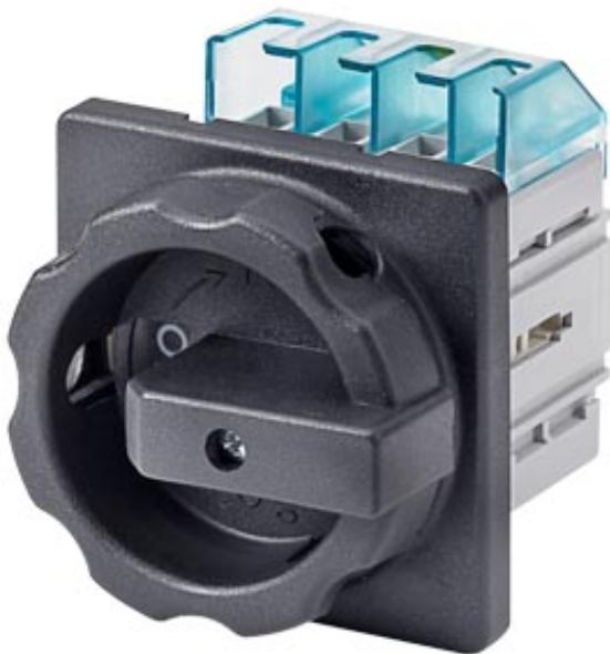
MASTER SWITCH 4-POLE IU=63, P/AC-23A W. 400V=22KW FRONT MOUNTING FOUR- HOLE MOUNTING ROT. MECHANISM BLACK
