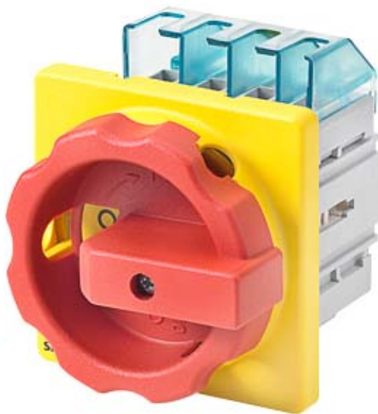
EMERG. STOP SWITCH 4-POLE IU=63, P/AC-23A AT 400V=22KW FRONT MOUNTING FOUR-HOLE MOUNTING ROTARY ACTUATOR RED/YELLOW (EMERG. STOP)
