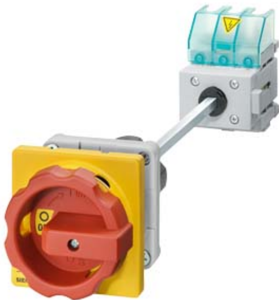
MAIN/EMERG. STOP SWITCH 3-POLE IU=125, P/AC-23A AT 400V=45KW FLOOR MOUNTING DIN RAIL/TWO-HOLE MOUNTING ROTARY ACTUATOR RED/YELLOW (EMERG. STOP)
