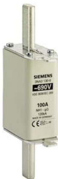
LV HRC FUSE LINK GL/GG WITH NON-INSULATED GRIP LUGS WITH FRONT INDICATOR SIZE 1, 100A, AC 690V/DC 440V
