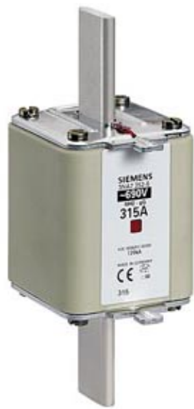
LV HRC FUSE LINK GL/GG WITH NON-INSULATED GRIP LUGS WITH COMBINATION INDICATOR SIZE 2, 315A, AC 690V/DC 440V
