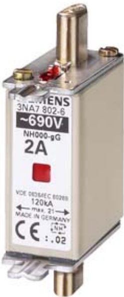
LV HRC FUSE LINK GL/GG WITH NON-INSULATED GRIP LUGS WITH COMBINATION INDICATOR SIZE 000, 2A, AC 690V/DC 250V
