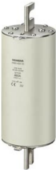
SITOR FUSE-LINK FOR SEMICONDUCTOR PROTECTION 315A AR 1500V SIZE 3 CONNECTION CONTACT INDICATOR 210MM
