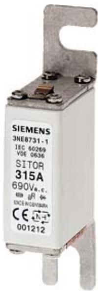
SITOR FUSE-LINK FOR SEMICONDUCTOR PROTECTION 315A AR, AC 690V, DC 700V SIZE 000, BRACKETS 80MM
