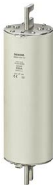
SITOR FUSE-LINK FOR SEMICONDUCTOR PROTECTION 125A AR 2500V SIZE 3 CONNECTION CONTACT INDICATOR 260MM
