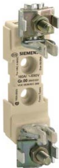
LV HRC FUSE BASE 690V(1000V) SINGLE-POLE,160A,SIZE 00 STRAIGHT-WIRE TERMI.2.2-50SQMM
