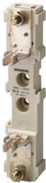
LV HRC FUSE BASE 690V(1000V) SINGLE-POLE, 160A, SIZE 0 PAD-TYPE TERMINAL
