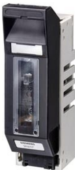
LV HRC FUSE BASE AC 690V WITH SLEWING EQUIPMENT SIZE 00 160A 1POLE W.SCREW-TYPE TERMINAL CONNECTION
