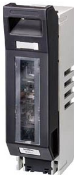
LV HRC FUSE BASE AC 690V WITH SLEWING EQUIPMENT SIZE 1 250A 1POLE W.SCREW-TYPE TERMINAL CONNECTION
