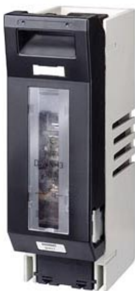
LV HRC FUSE BASE AC 690V WITH SLEWING EQUIPMENT SIZE 3 630A (SIZE 2 400A) 1POLE W.SCREW-TYPE TERMINAL CONNECTION
