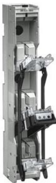
IN-LINE FUSE SWITCH DISCONNECTOR 3-POLE SWITCHABLE, SIZE 1, I=250A , U=690V, TERMINAL STUD M 10 NEW DESIGN
