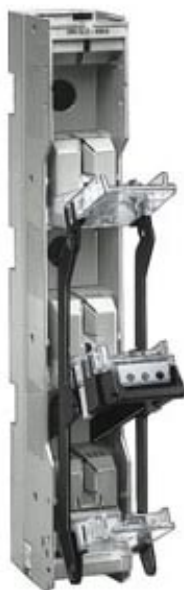
IN-LINE FUSE SWITCH DISCONNECTOR 3-POLE SWITCHABLE, SIZE 3, I=630A , U=690V, TERMINAL STUD M 12 NEW DESIGN
