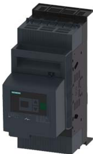
FUSE-SWITCH-DISCONNECTOR 3-POLE, NH000, 160A 40MM BUSBAR SYSTEM COVER LEVEL 32/70 MM BOX TERMINAL FUSE MONITORING ELECTRONIC, EFM 20
