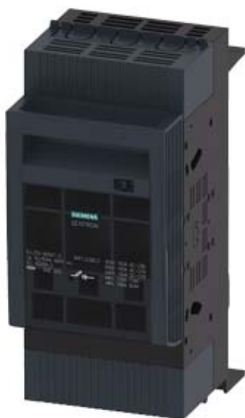
FUSE-SWITCH-DISCONNECTOR 3-POLE, NH000, 160A 60MM BUSBAR SYSTEM COVER LEVEL 32/70 MM BOX TERMINAL
