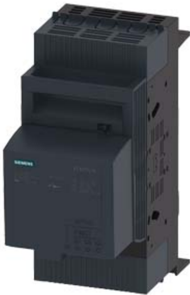
FUSE-SWITCH-DISCONNECTOR 3-POLE, NH000, 160A 60MM BUSBAR SYSTEM COVER LEVEL 32/70 MM BOX TERMINAL FUSE MONITORING ELECTRONIC, EFM 10
