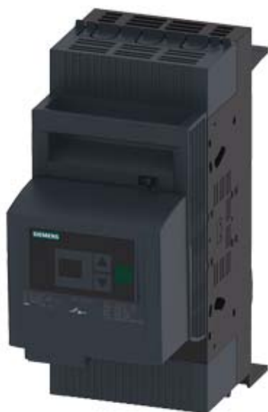
FUSE-SWITCH-DISCONNECTOR 3-POLE, NH000, 160A 60MM BUSBAR SYSTEM COVER LEVEL 32/70 MM BOX TERMINAL FUSE MONITORING ELECTRONIC, EFM 20
