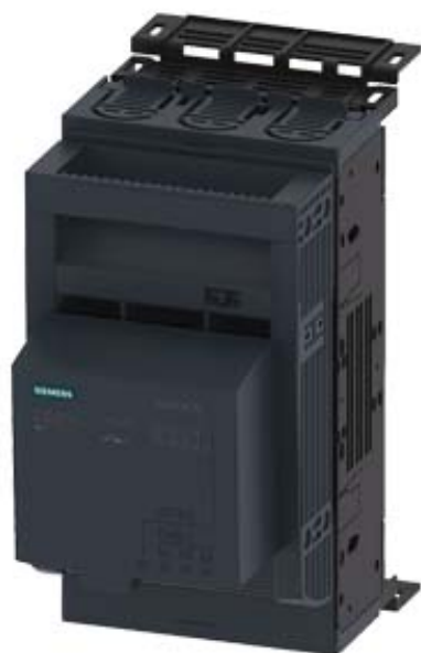
FUSE-SWITCH-DISCONNECTOR 3-POLE, NH00, 160A 40MM BUSBAR SYSTEM COVER LEVEL 32/70 MM FLAT CONNECTOR FUSE MONITORING ELECTRONIC, EFM 10
