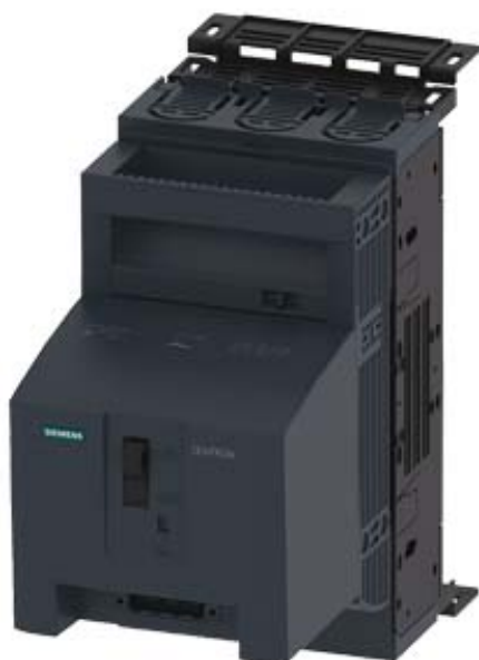
FUSE-SWITCH-DISCONNECTOR 3-POLE, NH00, 160A 40MM BUSBAR SYSTEM COVER LEVEL 32/70 MM BOX TERMINAL FUSE MONITORING ELECTROMECHANICAL
