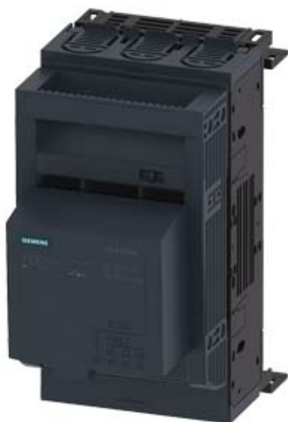
FUSE-SWITCH-DISCONNECTOR 3-POLE, NH00, 160A 60MM BUSBAR SYSTEM COVER LEVEL 32/70 MM FLAT CONNECTOR FUSE MONITORING ELECTRONIC, EFM 10
