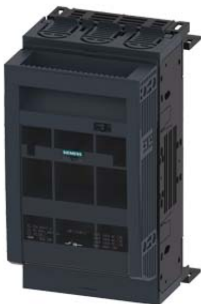
FUSE-SWITCH-DISCONNECTOR 3-POLE, NH00, 160A 60MM BUSBAR SYSTEM COVER LEVEL 32/70 MM BOX TERMINAL
