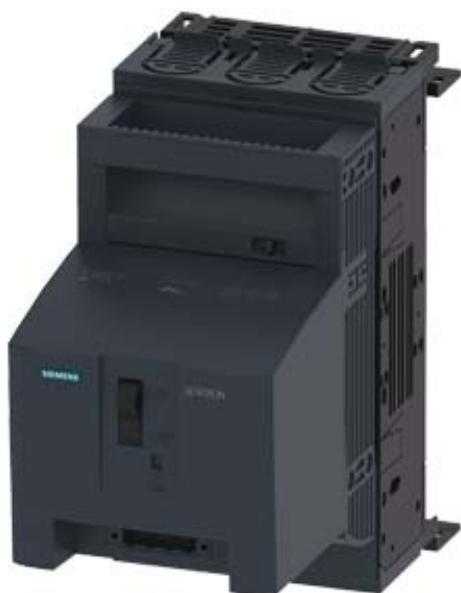
FUSE-SWITCH-DISCONNECTOR 3-POLE, NH00, 160A 60MM BUSBAR SYSTEM COVER LEVEL 32/70 MM BOX TERMINAL FUSE MONITORING ELECTROMECHANICAL
