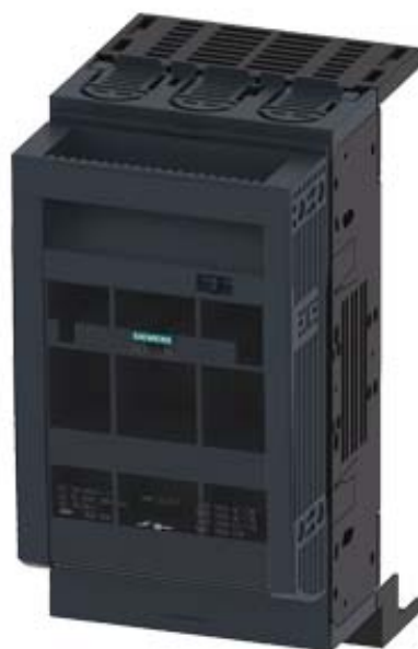
FUSE-SWITCH-DISCONNECTOR 3-POLE, NH00, 160A 60MM BUSBAR SYSTEM COVERS FOR RITTAL BOX TERMINAL
