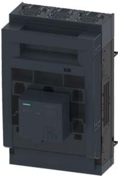
FUSE-SWITCH-DISCONNECTOR 3-POLE, NH1, 250A 60MM BUSBAR SYSTEM COVER LEVEL 32/70 MM BOX TERMINAL FUSE MONITORING ELECTRONIC, EFM 10
