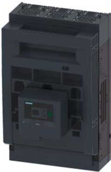
FUSE-SWITCH-DISCONNECTOR 3-POLE, NH1, 250A MOUNTING PLATE CONSTRUCTION COVER LEVEL 70 MM FLAT CONNECTOR FUSE MONITORING ELECTRONIC, EFM 20
