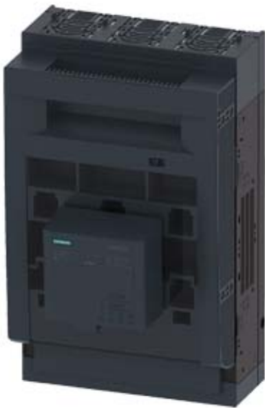
FUSE-SWITCH-DISCONNECTOR 3-POLE, NH1, 250A MOUNTING PLATE CONSTRUCTION COVER LEVEL 70 MM BOX TERMINAL FUSE MONITORING ELECTRONIC, EFM 10
